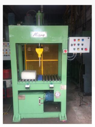
Micro Technical Team has designed and Developed rubber Bale Cutting Machine that is required in Rubber Industry for cutting of the rubber bales of various sizes The Machine comes manual Control and Push Button Control with Relay Logic. The Hardened Rollers are incorporated for the free movement of the Bale. These Machines are in H Frame Fabricated and The Tonnage Capacity is Up to 100 Ton.
