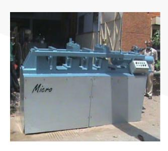
The Hydraulic Swaging Machine is put to use when the clients want to reduce the diameter of the solid rod or the pipe to a particular length. We manufacture different types of Hydraulic Swaging Machine to meet the requirement of our clients. With the help of this machine a pipe as well as rod, both can be swaged. When you are using our products, you will enjoy certain advantages like:
