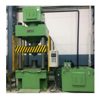
Cold forging Process is defined as forming or forging of a bulk material at room temperature with no initial heating of the preform or inter- mediate stages. Cold extrusion is a special type of forging process wherein the cold metal flows plastically under compressive forces into a variety of shapes.
