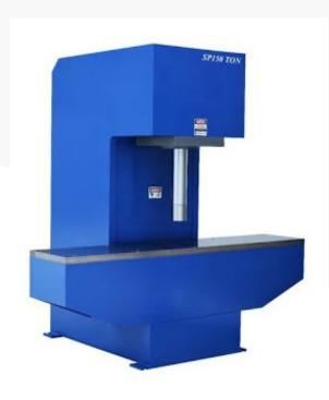
Straightening is the Key requirement in Components of Auto Industry & General Industry , Components get deformed after being processed and the same has to be Straighten by removing the deformation in work piece with respect to the requested tolerances
