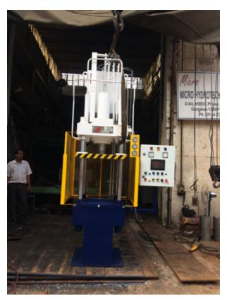
The Trimming Presses are used for demurring the flashes in castings of Aluminum, Magnesium and Zinc as shown in Images, which are casted from High Pressure Die Casting Machine (HPDC) and Gravity Die Casting Machine. As it is not Practical to Machine the Flashes therefor to debur the Flashes Micro Has Designed and Developed a Hydraulic Trimming Press Machine Solution to Remove the Flashes.
